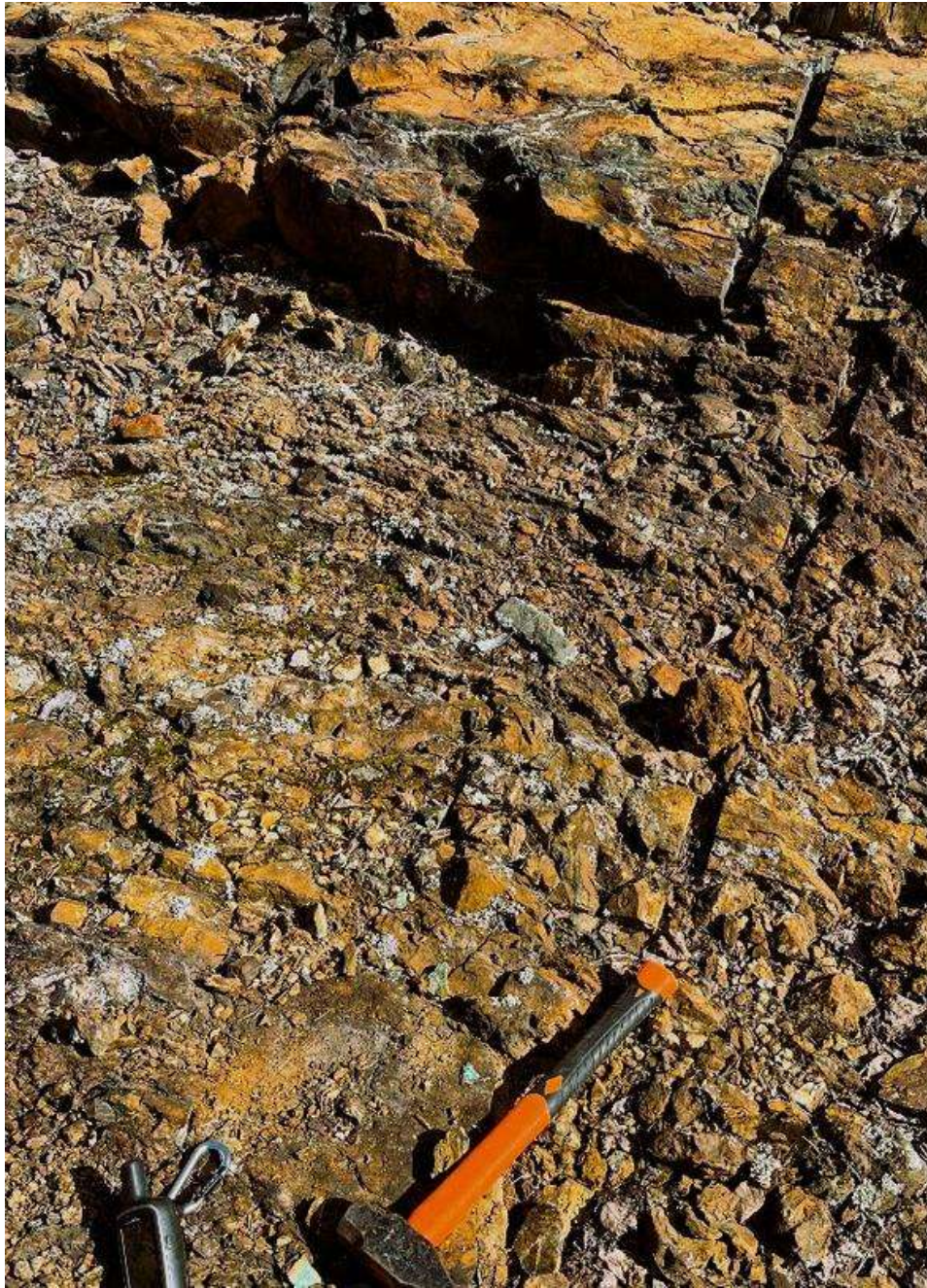
Oxidized volcanics in sample A0284709 returned 2.48% Cu and 1.215 g/t Au
