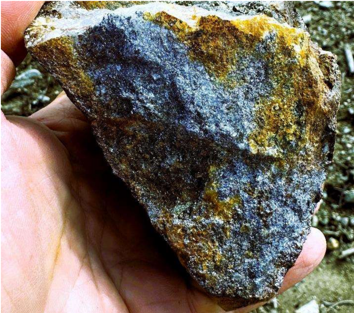
Sample A0284675 showing Molybdenite covered fracture
