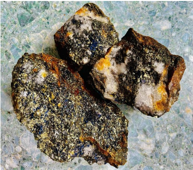
Sample A0284675 with coarse Chalcopyrite, Bornite, and Molybdenite (11.35% Cu, 0.17% Mo, 1.55 g/t Au, and 129 g/t Ag)
