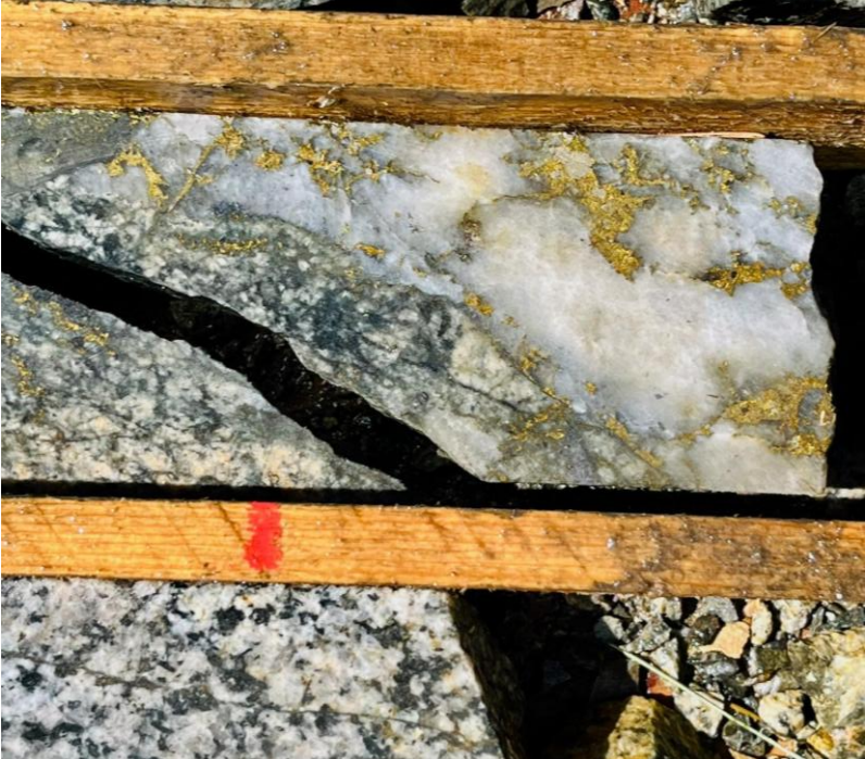
IS06-03 sample is from 103.2m to 106.1m which ran 1.1% CuEq over 3.09m, including 5.68% CuEq over 0.22m
