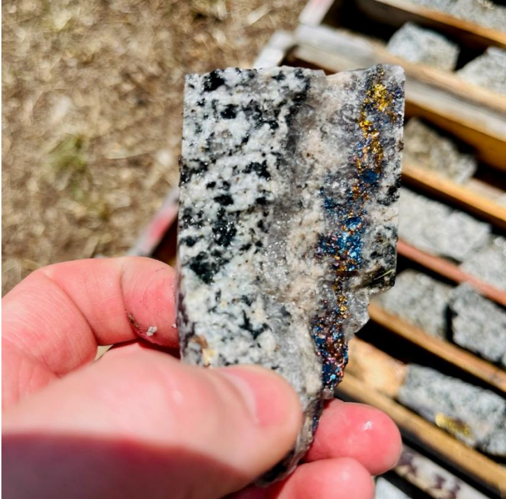
IS08-54 sample is from 178.91m to 184.05m which ran 1.07% CuEq over 5.14m, including 2.45% CuEq over 0.96m
